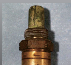
Ethylene Glycol (Antifreeze) Contamination
