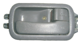
200-201-045 Hiace94-2000 front door handle HIACE 94-95 69278-95J00-03 LH 69277-95J00-03 RH 69278-95J00-B0 LH 69277-95J00-B0 RH
