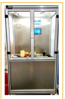
Bubble test bench to test the integrity of the oil filter element, and the maximum aperture and average aperture of the filter paper.
