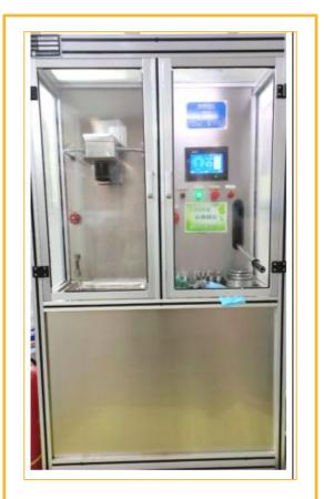
Anti drain back valve bench to test the sealing
