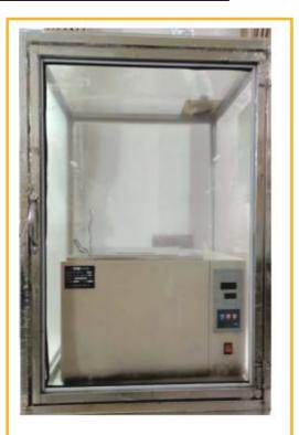
High oil temperature resistance test tank to test high oil temperature resistance of products and parts
