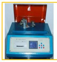
Electronic stiffness tester to test the tension generated by bending filter paper at a certain angle
