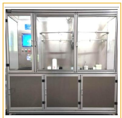
Flow resistance test bench to test filter rated flow resistance and bypass valve opening pressure.
