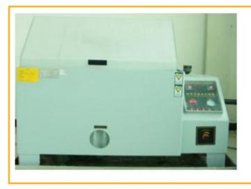
Salt spray corrosion test machine to test material corrosion resistance
