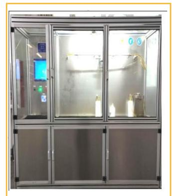
Fuel filter integrated test bench to test cleaness and pressure drop flow characteristics.
