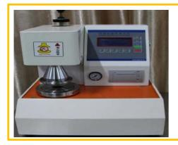
Paper breaking resistance tester to test the strength of filter mdeia/ paper under pressure
