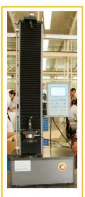
Automatic spring testing machine to test spring compression and tensile
