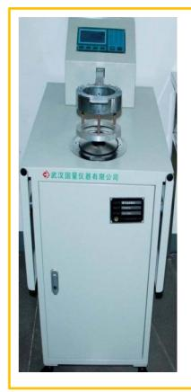
Air permeability tester to test filter media/paper air permeability
