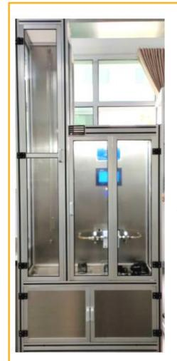
Pressure test bench to test the pressure when the filters are destroyed.
