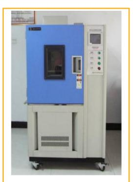
High and low temperature alternating humid heat test chamber to test the performance of filter and filter parts at high temperature150°C or low temperature -40°C
